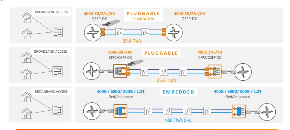
Reduce Power, Space with Pluggables, Reduce Cost/Bit/Km with Embedded
