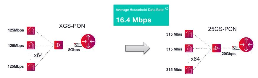
With service provider deploying XGS-PON with an easy evolution to 25GS-PON the access will be able to support the existing and future application for years
